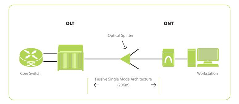
The Optical Line Terminal (OLT) resides in the Data Centre or core network. It connects to the core switch using traditional Ethernet core connectivity.
