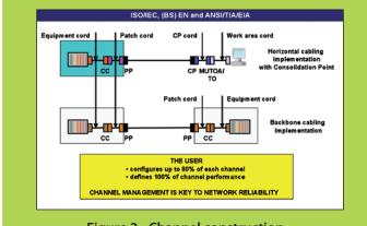
Figure 2 - Channel construction
